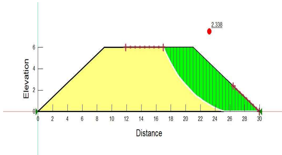
Figure 5.2(1.1) Morgenstern-Price method factor of safety
