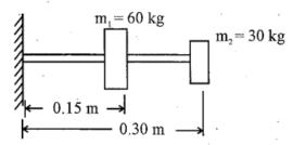
Take E =  $2 \times 10^{11}$  N/m<sup>2</sup> and cross section moment of inertia of the beam I =  $4 \times 10^{-7}$  m.
