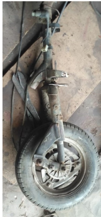
Figure 4.6: Steering during fabrication
