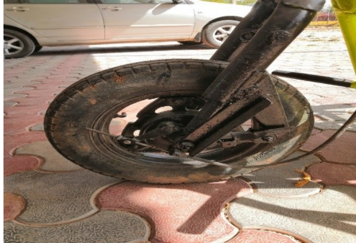
Figure 4.9: Drum Brakes used in vehicle
