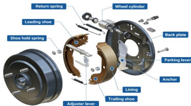
Figure 4.8: Various parts of drum brake
