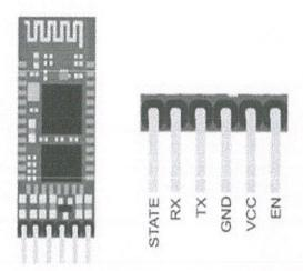
It is a small portable device that is used to be connected in the Arduino board so that it can communicate with mobile or smartphone.
