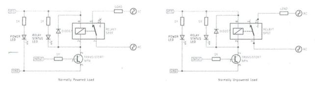
For simple on/off applications, the relay can be connected as shown above. One terminal of mains is connected to common, and the other is connected to NO or NC depending on whether the load should be connected/disconnected when the relay is active.
