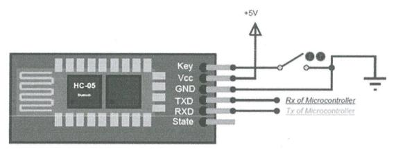
During power up the key pin can be grounded to enter into Command mode, if left free it will by default enter into the data mode. As soon as the module is powered you should be able to discover the Bluetooth device as "HC-05" then connect with it using the default password 1234 and start communicating with it. The name password and other default parameters can be changed by entering into the
