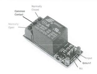
Relay is an electromechanical device that uses an electric current to open or close the contacts of a switch. The single-channel relay module is much more than just a plain relay, it comprises of components that make switching and connection easier and act as indicators to show if the module is powered and if the relay is active or not.
