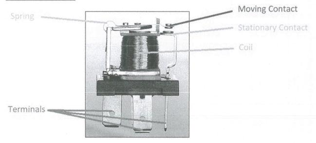
The relay uses an electric current to open or close the contacts of a switch. This is usually done using the help of a coil that attracts the contacts of a switch and pulls them together when activated, and a spring pushes them apart when the coil is not energized.
