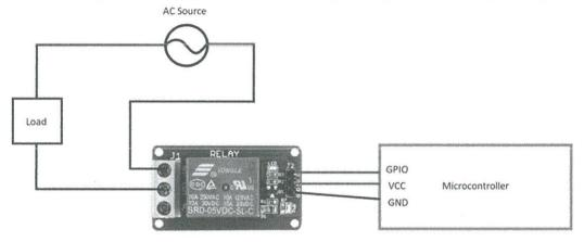
The mains wiring is screwed to the terminal block, and the microcontroller can be connected using jumper cables.
