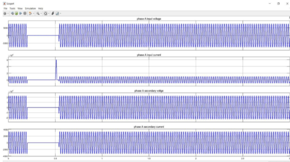
Figure 4.6: Phase A(Primary and Secondary Voltages and Currents)
