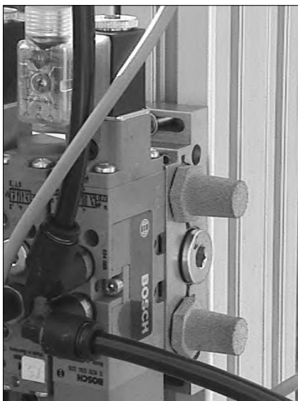
Fig. 8a: Valves mounted to T-slot
