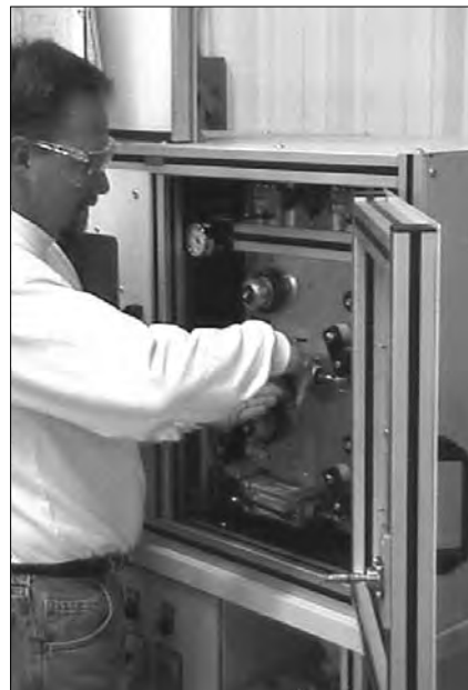
Fig. 7: A lean cell constructed from modular aluminum framing provides for easy maintenance and repair
