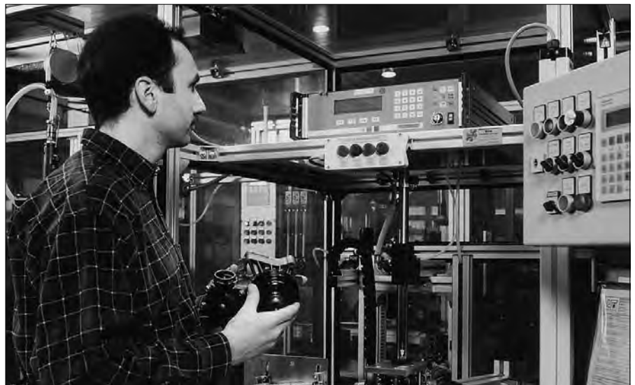
Fig. 6: Visual Inspection verifies parts are correctly assembled and function properly.
