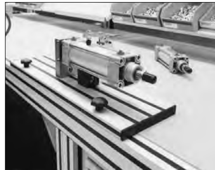
Fig. 5a: Quick change fixture
