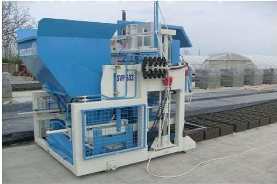
Fig. 2 Movable Concrete Automatic Machine
