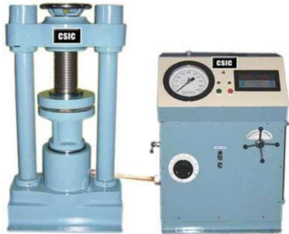
Fig: Compressive Strength Test on Concrete
