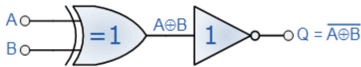
2-input "Ex-OR" gate plus a "NOT" gate
