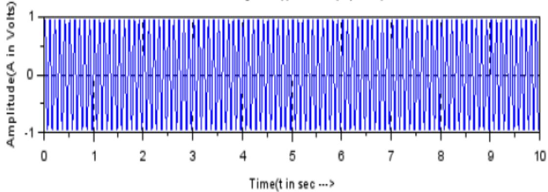
$$\text{AM-DSB/FC Modulated signal: } s(t) = (1 + m(t)) \cdot c(t)$$
