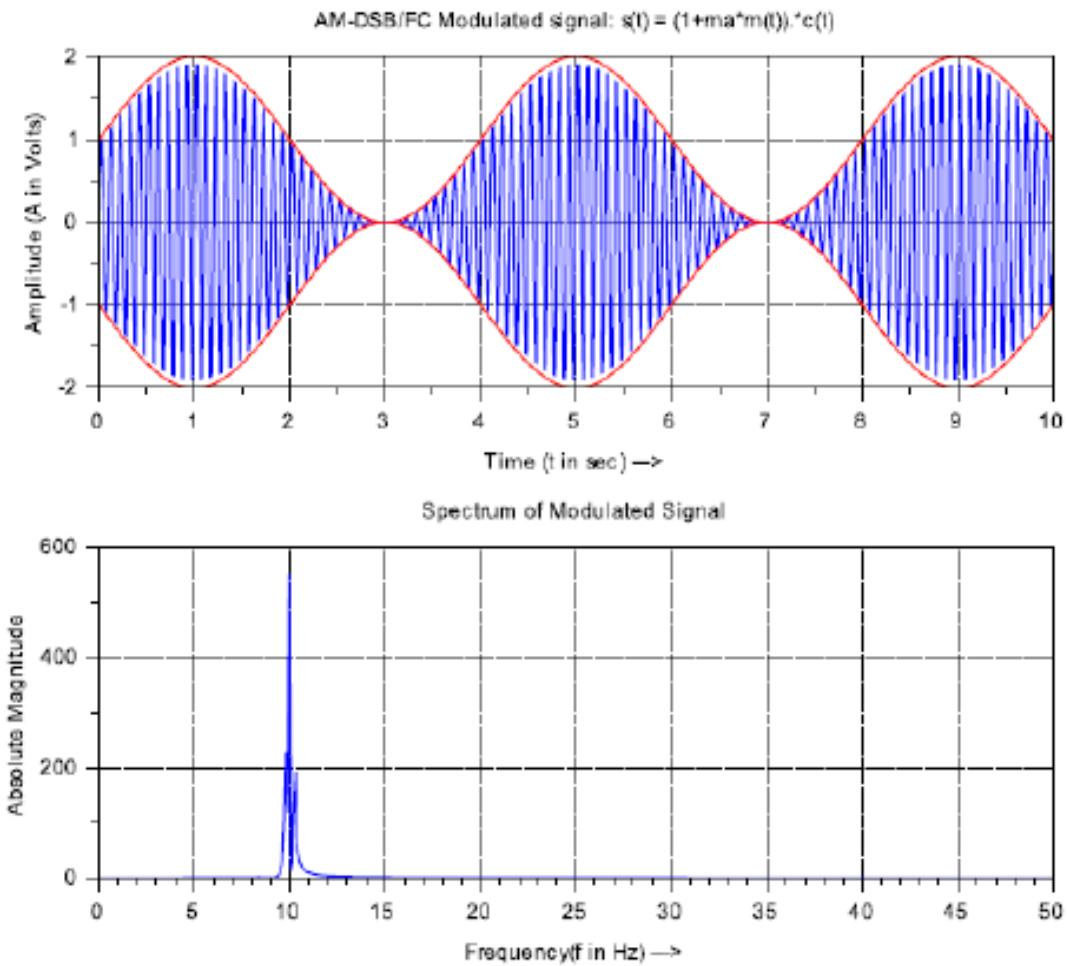
**Exp.3- Matlab Code to generation AM wave for different value of modulation index
