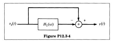
Sketch  $V(\omega)/V_s(\omega)$ . What is the corresponding cutoff frequency?
