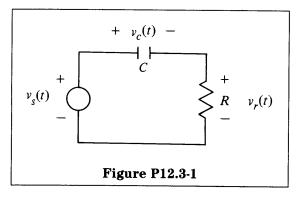
(a) Determine  $H_1(\omega)$ , the transfer function from  $v_s$  to  $v_c$ , as shown in Figure P12.3-2. Sketch the magnitude and phase of  $H_1(\omega)$ .
