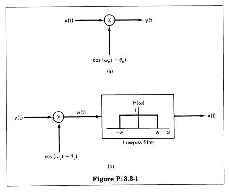
Let us denote the frequency difference between the modulator and demodulator as  $\Delta\omega$  [i.e.,  $(\omega_d - \omega_c) = \Delta\omega$ ]. Also, assume that x(t) is bandlimited with  $X(\omega) = 0$  for  $|\omega| \geq \omega_M$  and assume that the cutoff frequency W of the lowpass filter in the demodulator satisfies the inequality
