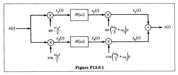
Sketch the Fourier transform of  $s_1(t)$ ,  $s_2(t)$ ,  $s_3(t)$ ,  $s_4(t)$ ,  $s_5(t)$ ,  $s_6(t)$ , and y(t), thus showing that y(t) is x(t) single-sideband-modulated on the carrier  $\omega_c$ . Assume that x(t) has the real Fourier transform shown in Figure P13.6-2 and that  $H(\omega)$  is a low-pass filter as shown in Figure P13.6-3.
