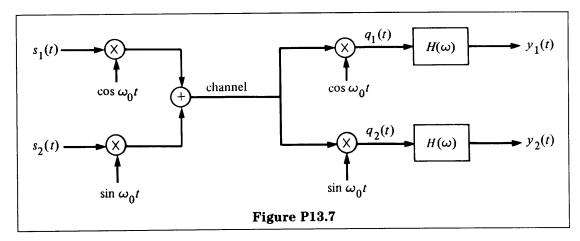
For  $y_1(t)$  to be the same as  $s_1(t)$ , and  $y_2(t)$  to be the same as  $s_2(t)$ , choose the proper filter  $H(\omega)$  and place the proper restrictions on the bandwidth of  $s_1(t)$  and  $s_2(t)$ .
