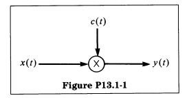
In the amplitude modulation system in Figure P13.1-1, the input x(t) has the Fourier transform shown in Figure P13.1-2.
