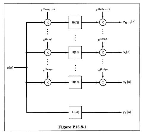
(b) Again with  $H(\Omega)$  as in Figure P15.8-2 and with  $\Omega_i = 2\pi i/N$ , determine the value of  $\Omega_0$  in terms of N so that the filter bank covers the entire frequency band without any overlap.
