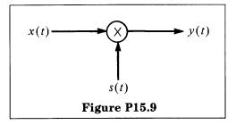
Suppose we know that  $X(\omega)$  is bandlimited to  $\pm \omega_c$  and that s(t) is an *arbitrary* periodic function with period *T*.
