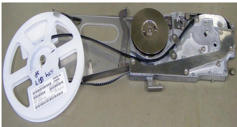
Fig.2: Tape-and-reel feed mechanism used to load components into a pick-and-place machine
