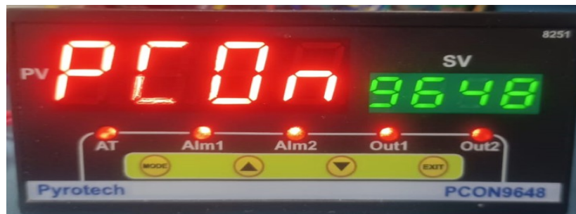
7 SEGMENT LED DISPLAY , LEDS & SWITCHES
