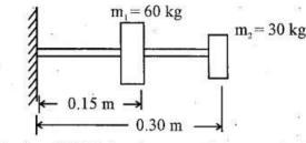
Take E =  $2 \times 10^{11}$  N/m<sup>2</sup> and cross section moment of inertia of the beam I =  $4 \times 10^{-7}$  m.
