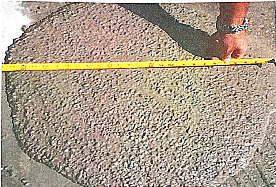
Fig. 3.2 T50 cm test procedure
