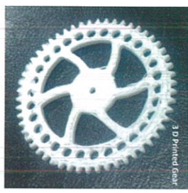
3D Printed Gear
